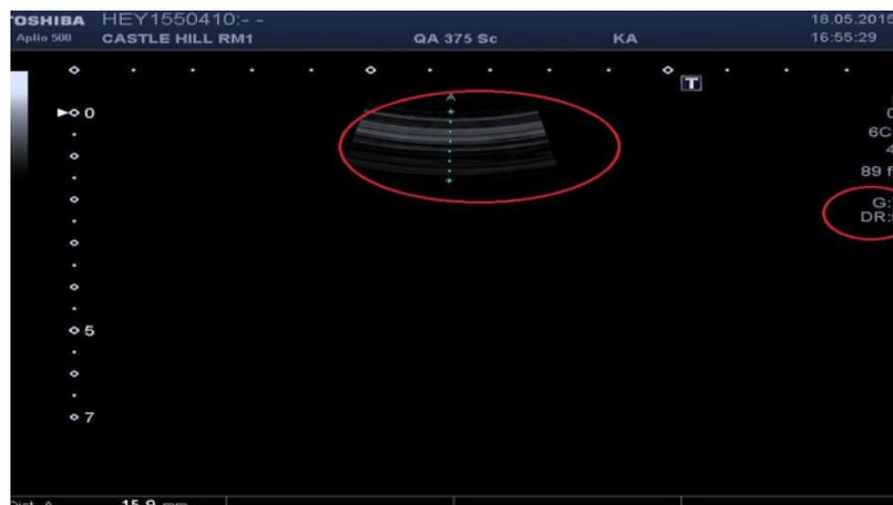
**Figura/Figure 2:** Teste de ruído eletrônico/Electronic noise test: The noise is highlighted in the indicated circle. Fonte/Source: BMUS guidelines for the regular quality assurance testing of ultrasound scanners by sonographers (Dudley, N *et al* 2014).
