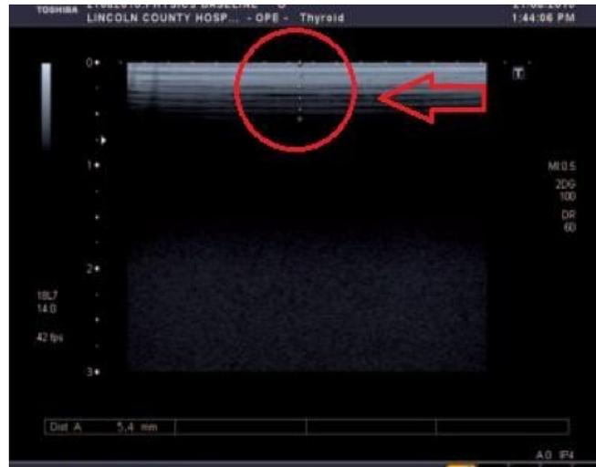
**Figura/Figure 1:** Teste de reverberação de ar/Air reverberation test: the reverberation lines cannot occupy more than 25% of the image depth according to the arrow and indicator circle. Fonte/Source: BMUS guidelines for the regular quality assurance testing of ultrasound scanners by sonographers (Dudley, N *et al* 2014).
